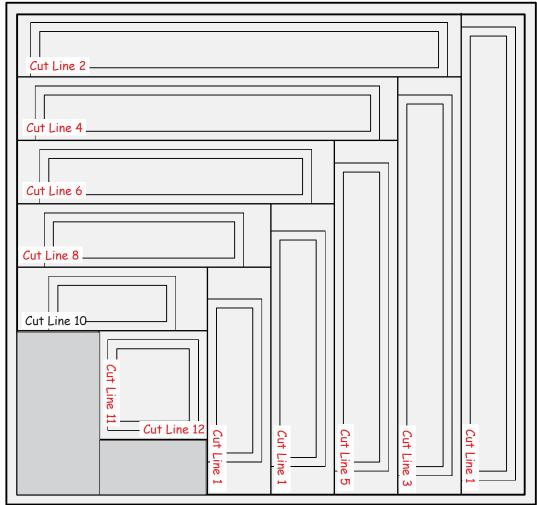
Cut Lines were all labeled Cut Line 10, but need to be Cut Line 1-12 as shown
